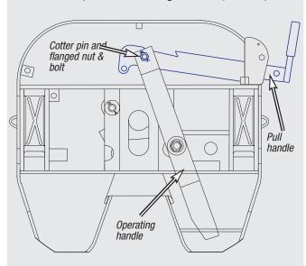
Attach the jaw spring to the jaw and the double springs to the pull handle. It is easier to attach the double springs to the handle first and then the clip.
