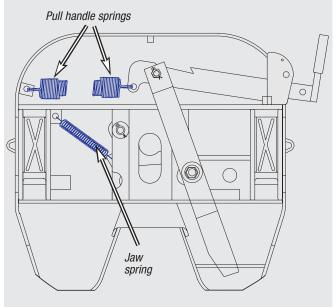
Remove the hex head flanged bolt and flanged nut assembly (items 10, 13 & 21) which secures the pull handle (item 18) to the operating handle (item 19).
