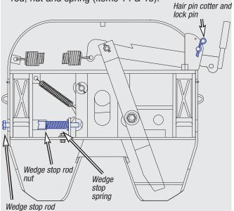
Remove the wedge stop rod guide (item 2) from rear cross member (2 bolt assemblies, items 20 & 22).
