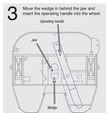
Attach the operating handle to the wedge assembly using a new socket bolt assembly (items 5, 6, 7, & 8). Position the operating handle over the hole in top plate to reach the socket from the other side.
