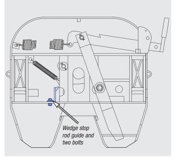
Remove the jaw spring (item 4) and pull handle springs (item 3) (smaller spring encased in larger spring to act as one spring).
